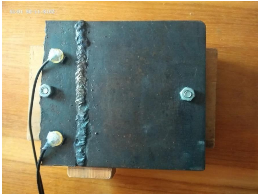
Figure 5.7 - Fixation of natural oscillations of the first plate by means of the emitter "white noise" and the receiver
