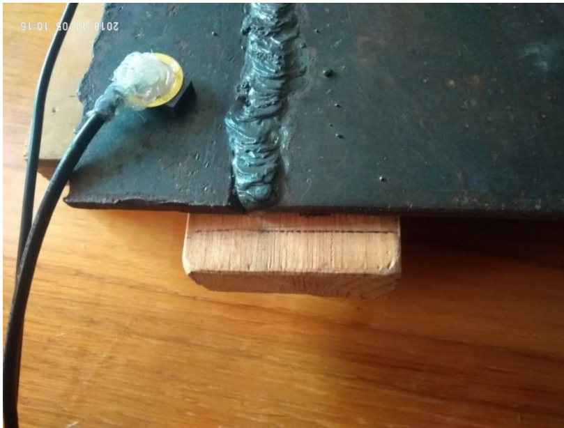
Figure 5.10 - Adjusting the impact force on the tested welded joint
