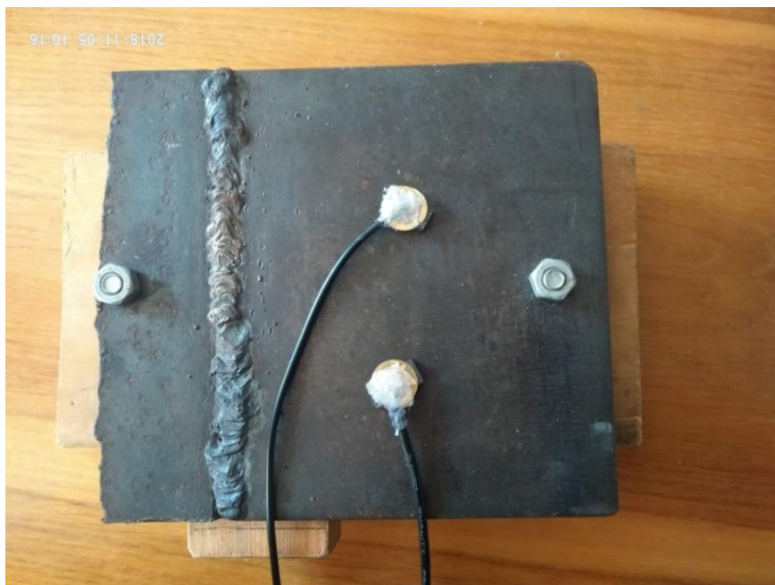
Figure 5.8 - Fixation of natural oscillations of the second plate by means of the emitter "white noise" and the receiver
